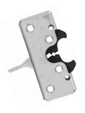
This two rotor latch is a sub-platform to the Tri*Mark* proven 050-0100 series latch and is designed for medium to heavy-duty applications for on or off-higway entrance doors, compartments and access panels. It features an internal trip mechanism for applications where it is desirable to have the release mechanism inline with the latch and a single position latch.
